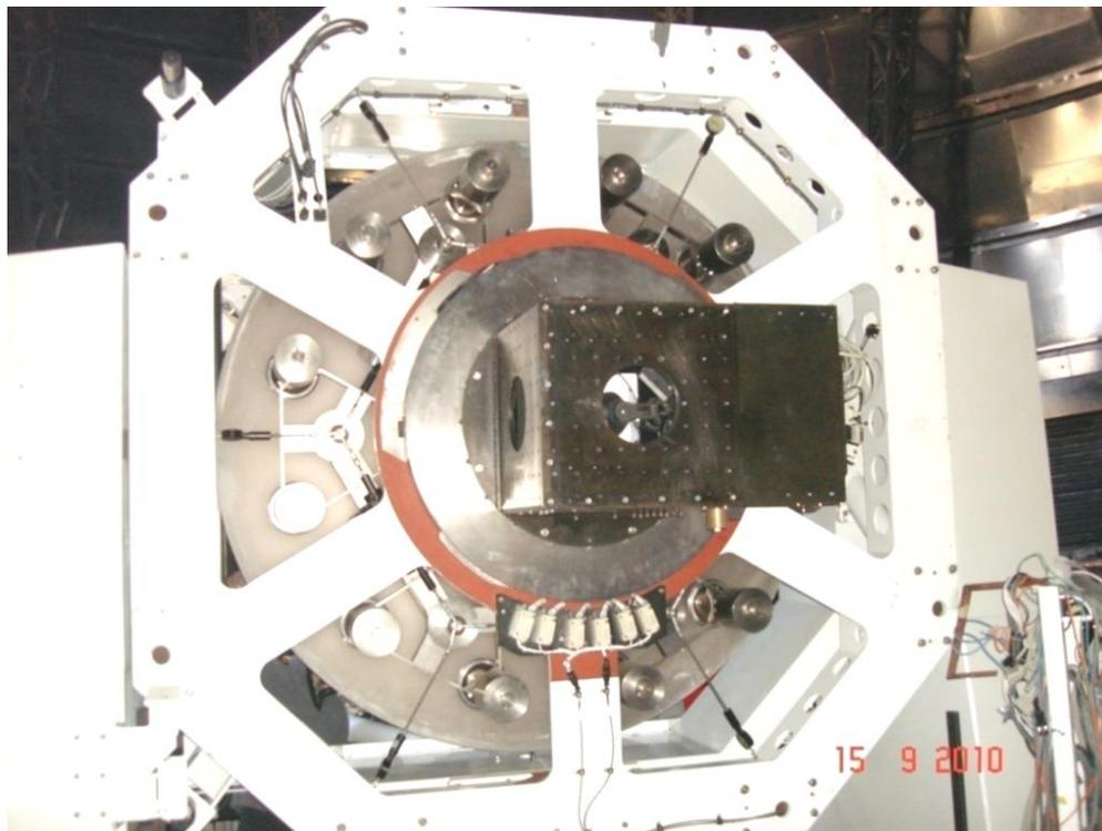
**Fig 1. : Whiffle tree mirror support system.**
