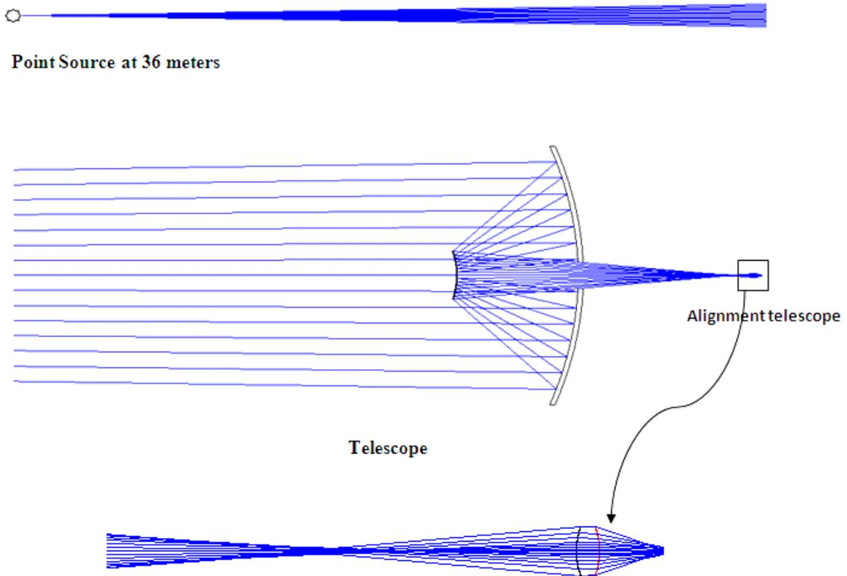
**Fig: 8: Alignment of the Telescope Optics**
