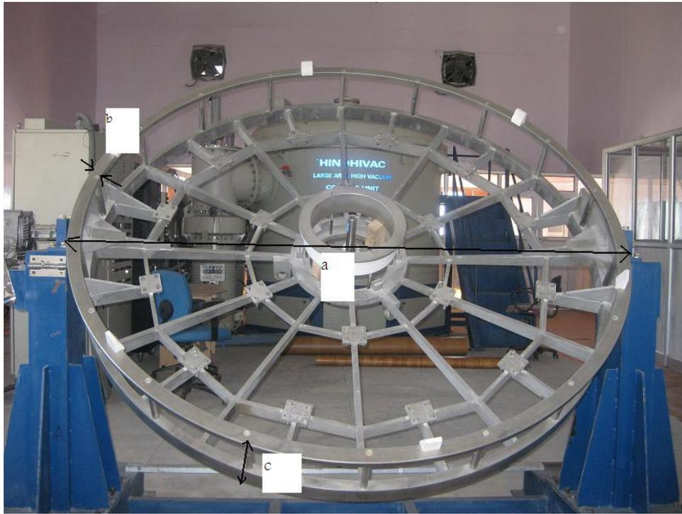
**Fig 7: Tilting Fixture & Rotation Mechanism**
