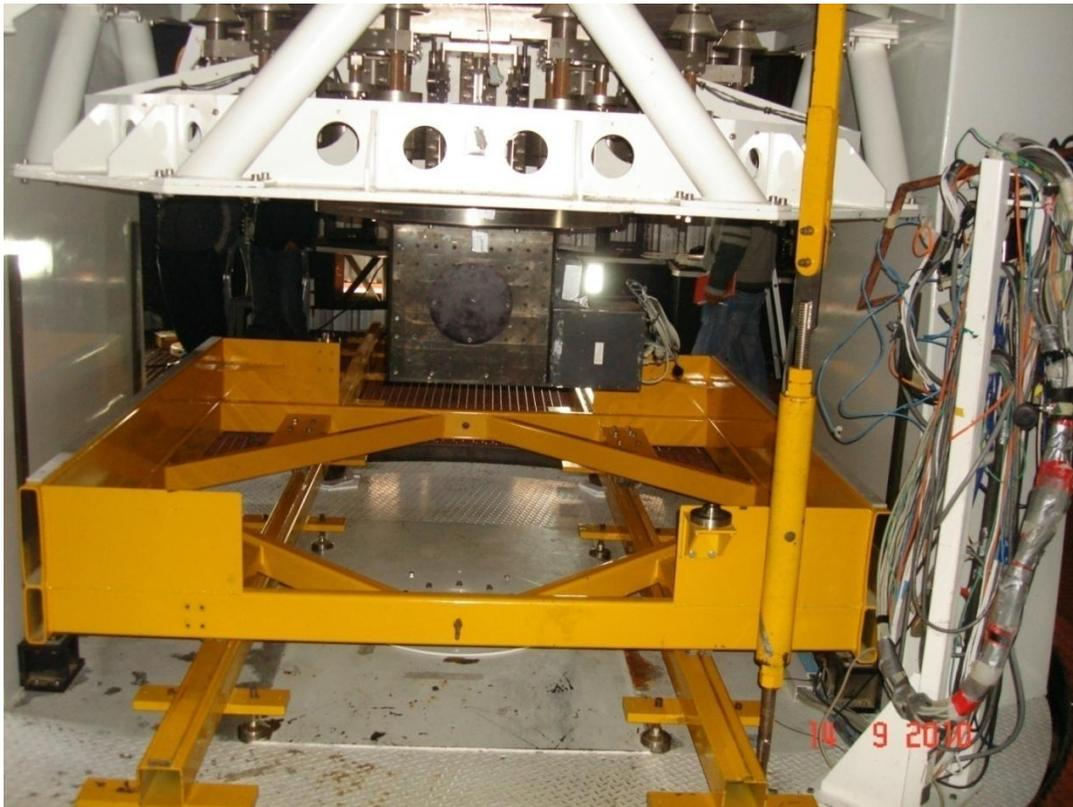
**Fig 5b. Mirror cell lowering over EOST cart.**
