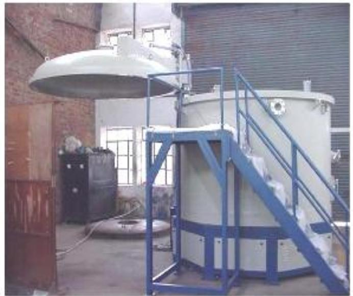
**Fig 4: 2.5M diameter vacuum coating plant.**
