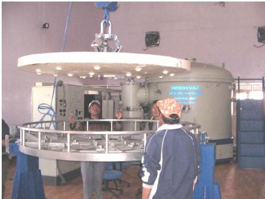
**Fig 3a: Integration of dummy mirror with tilting mechanism**
