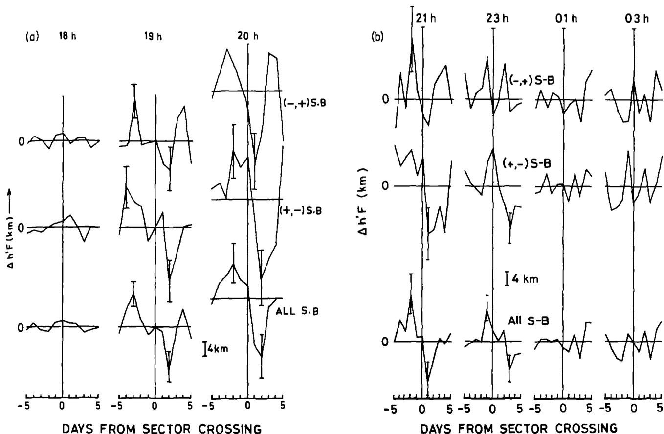
FIG. 1. (a) Average patterns of  $h'F$  at Kodaikanal for 1800, 1900, and 2000 LT derived from a superposed epoch analysis with respect to solar magnetic sector boundary crossings of type (+, -), (-, +) and all sector boundaries. A total of 73 sector boundaries observed over the periods 1957–1959 and 1968–1970 are used in the analysis. (b) Same as in (a), but for local time 2100, 2300, 0100, and 0300 h.
