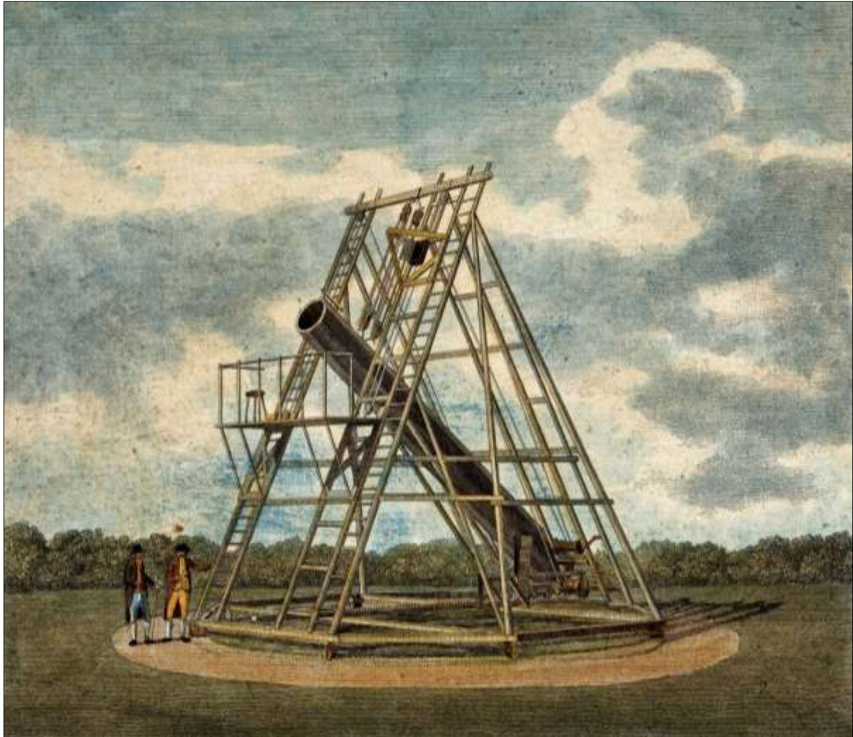
Figure 6: "Astronomy: a 40-ft telescope constructed by William Herschel, in use outdoors. Coloured etching, 18--. Wellcome Collection." (Reference: 46257i, https://wellcomecollection.org/works/srz5zy9y ).
