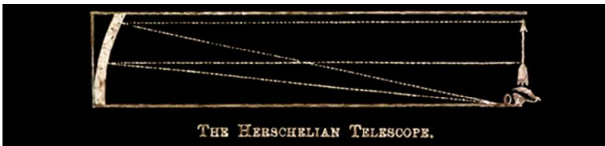
Figure 7: The Herschel telescope (after Chambers, 1877: 609 ).
