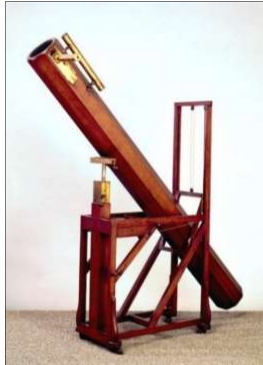
Figure 8: The 7-ft reflecting telescope by William Herschel, 1783–1785, in the collection of the Science Museum in London ( https://collection.sciencemuseumgroup.org.uk/objects/co56255/reflecting-telescope-by-william-herschel-1783-1785-telescope-newtonian-telescope-reflecting CC BY-NC-SA 4.0).
