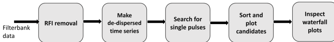
Figure 5.1: Single pulse search pipeline
