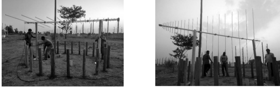
Figure A.6: Radiation pattern measurement for E-plane (Left) and H-plane (Right)
