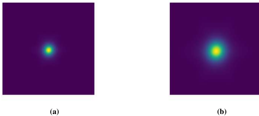
Figure 2.4: Long exposure PSFs of one lenslet as the wavefront propagates through different layers of the atmosphere. (a) After passing through the layer at 2 km. (b) After passing through the layer at 1 km.
