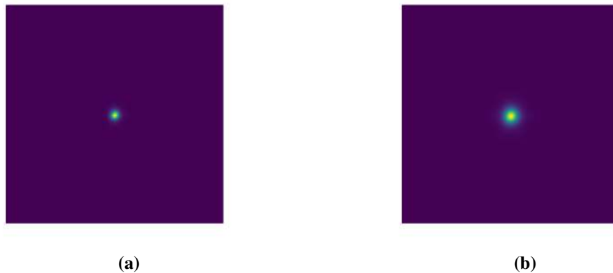
Figure 2.3: Long exposure PSFs of one lenslet as the wavefront propagates through different layers of the atmosphere. (a) After passing through the layer at 4 km. (b) After passing through the layer at 3 km.
