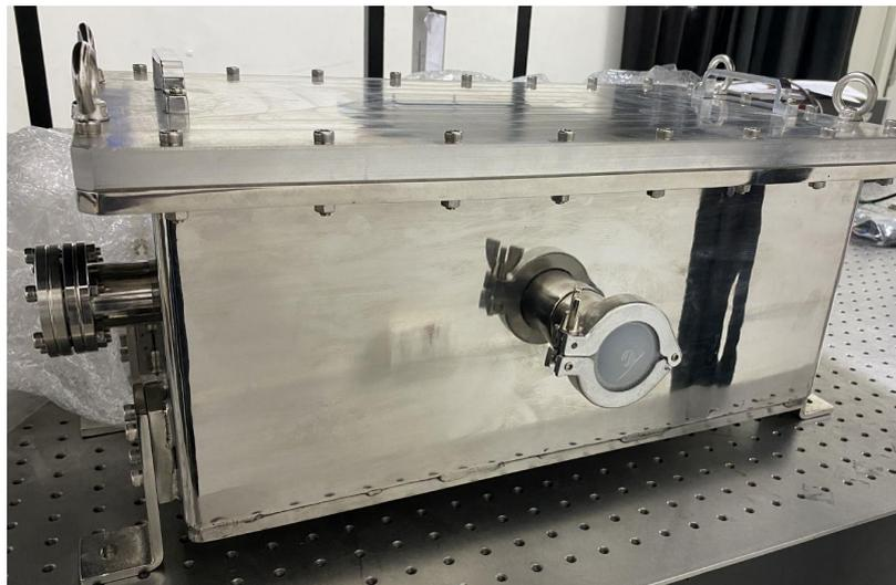
**Figure 7.1:** The new rectangular vacuum chamber that will be used for future upgradation of the instrument.
