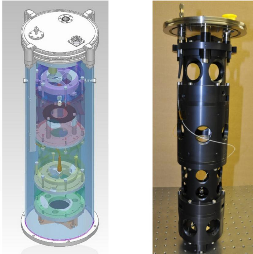
**Figure 2.10:** Opto-mechanical design of the FP calibrator for HARPS. The image on the left shows the CAD view. The right image is the assembled enclosure with FP and related optics inside, along with the optical fibers. Credits: Wildi *et al.* (2012)
