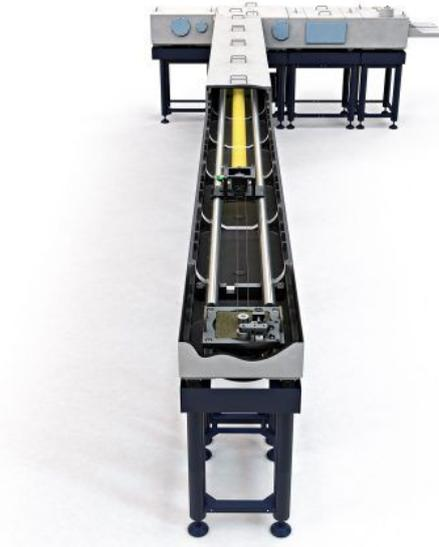
**Figure 5.2:** Bruker IFS 125HR Fourier Transform Spectrograph. Credits: Bruker Optics
