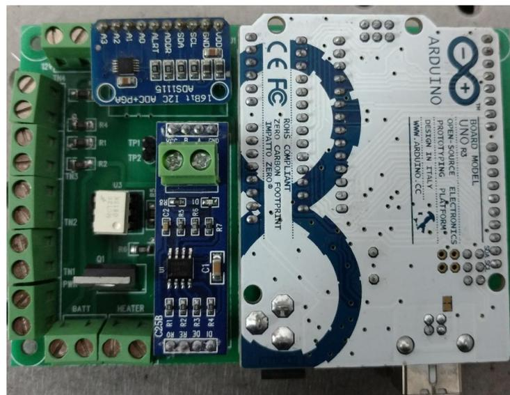
**Figure 4.6:** Temperature controller circuit with Arduino Uno Microcontroller.
