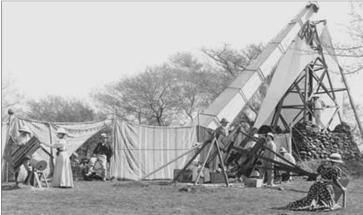
Figure 39: A scene showing the Lick Observatory party ready for the eclipse. All of the instruments are in place and the volunteers are at their practice stations. The 40-ft Schaeberle Camera with its twin wooden towers dominates the scene (courtesy: Mary Lea Shane Archives).
