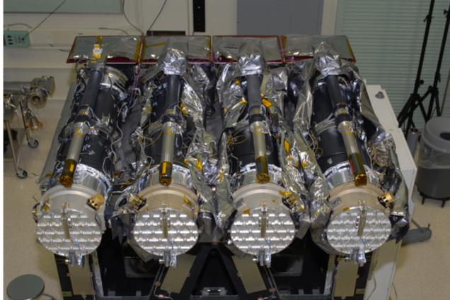
FIGURE 2.2: A view of the four telescopes on-board the SDO. *Image credits :* (Lemen et al. 2011)
