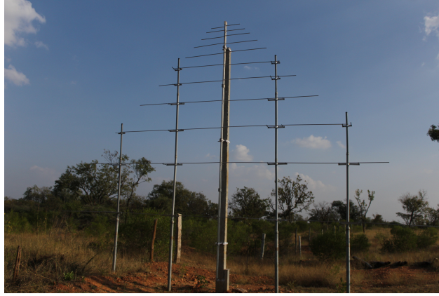
Figure 2.3: The 15 - 85 MHz LPDA (foreground) in the field. This longest dipole arm of this antenna is 500 cm. The height of the antenna is 5.2 m.
