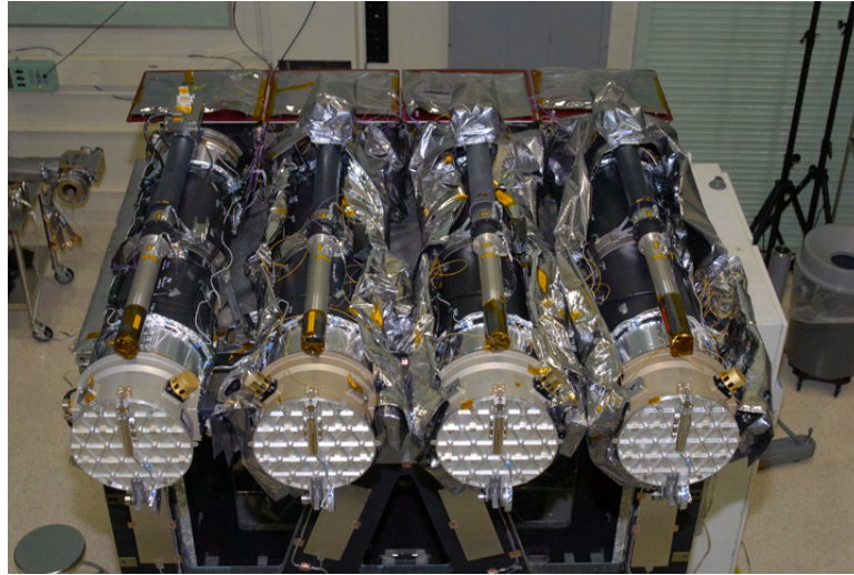
Figure 2.2: The array of four AIA telescopes mounted on the SDO spacecraft. Credit: Lemen et al. (2012)
