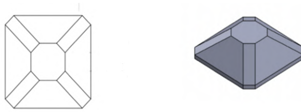
Figure 5.3: An illustration of exaggerated tip and edge of a deformed pyramid
