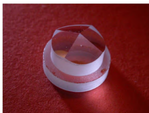
Figure 5.2: Image of a Pyramid wave-front sensor courtesy of INAF - Osservatorio Astrofisico di Arcetri, Italy.
