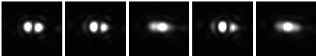
Figure 4.20: Experimental Narrowband PSF's for Red laser of 650 nm
