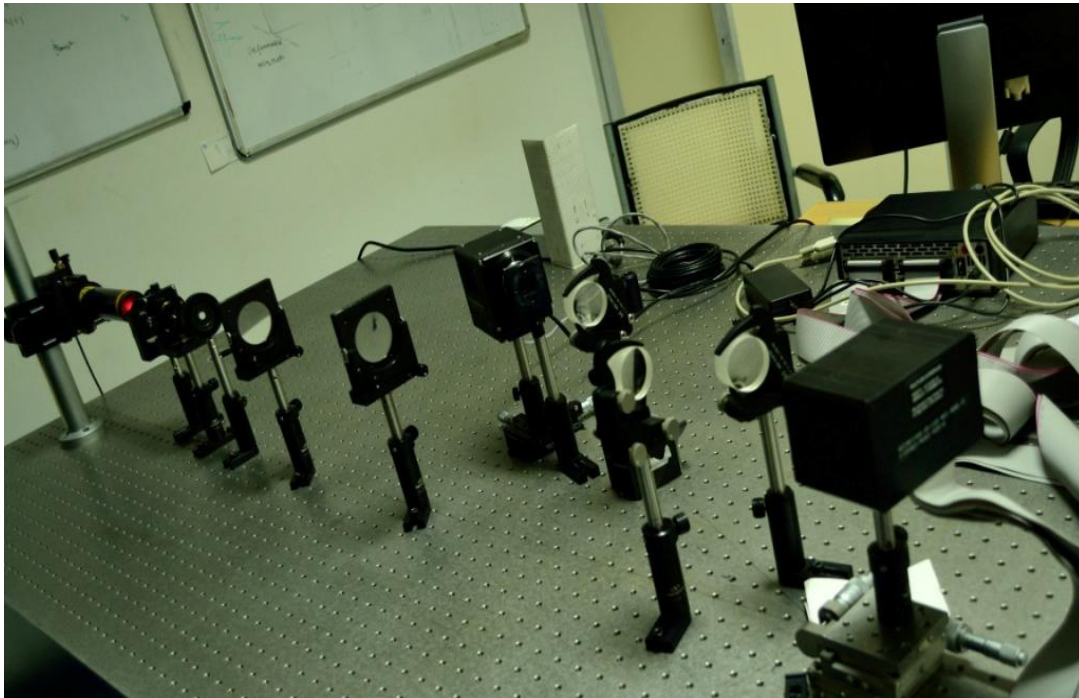
Figure 3. 3: Experimental setup for wave-front compensation
