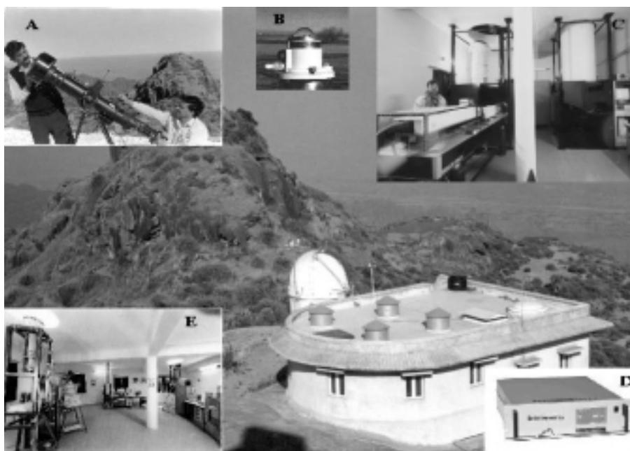
**Figure 1.** Panoramic view of the atmospheric sciences laboratory at Gurushikhar and the instruments: (A) All Sky Imaging (B) UV Radiometer (C) Inside View of Lidar Laboratory (D) Ozone Analyzer and (E) Inside View of Optical Aeronomy Laboratory.
