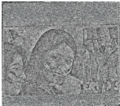
Figure 6. Image I_\phi reconstructed using only the phase information. The amplitudes for all Fourier components have been set equal to a fixed average value.
