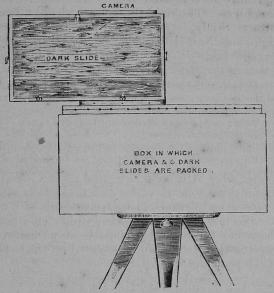
The shutter of the dark slide being in two pieces, the exposing of half the plate at a time is not difficult. Now move the camera 1½ inches from the centre to the right, and insert the left end of the dark slide, and expose, due care being taken that both exposures are the same. Prints from negatives so taken require no transposing, and can be trimmed and mounted without being divided.
