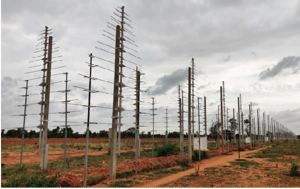
Figure 4.6: LPD antennae seen in the foreground were installed recently as part of GRAPH augmentation project. The individual dipoles in each LPD antenna are oriented along 0^\circ (Celestial North is the reference). Antennae noticed in the background are oriented along 90^\circ and they are part of the existing GRAPH.
