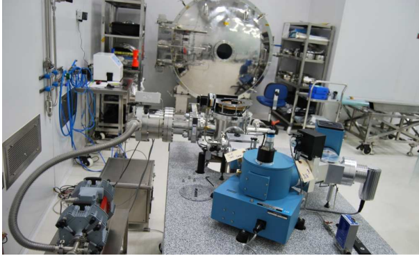
Figure 5.3: FUV-VIS Spectrophotometer facility
