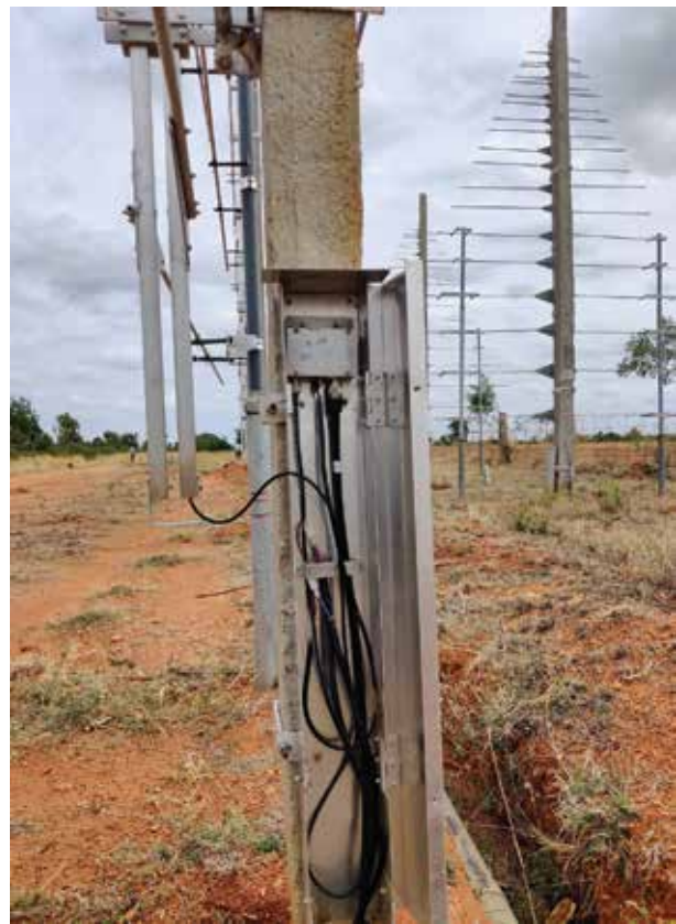
Figure 4.7: GRAPH augmentation project: Close-up view of the LPD antennas in mutually orthogonal orientation and the front end modules.
