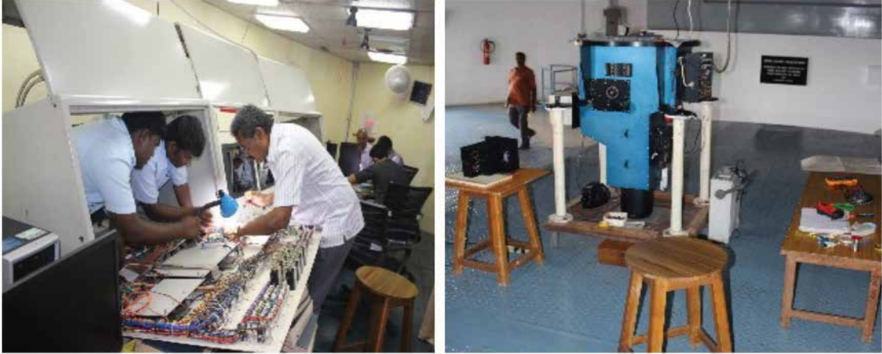
Figure 4.5: Wiring of the VBT console and replacement of the damaged components of the OMR spectrograph.
