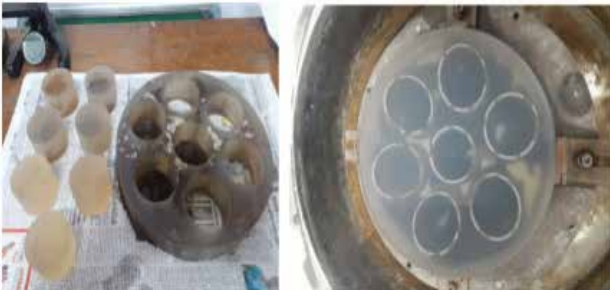
Figure 5.13: Left: Six glass blanks trepanned from parent glass blank using core drilling machine. Right: Curve generated parent glass blank with six mirror segments.
