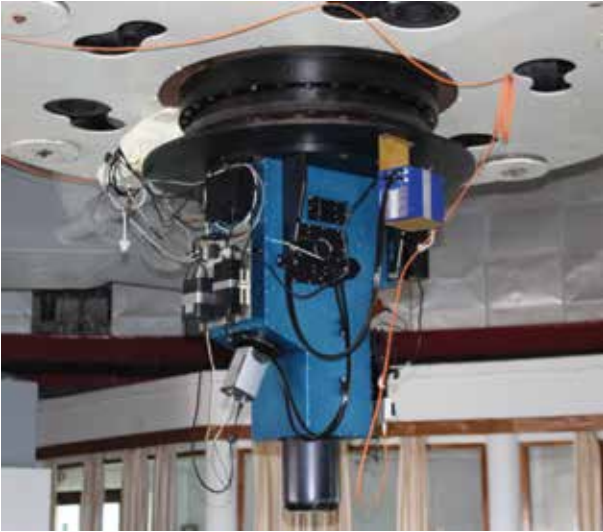
Figure 4.6: A new thermoelectrically cooled CCD Andor Newton DU920P attached with the OMR spectrograph.
