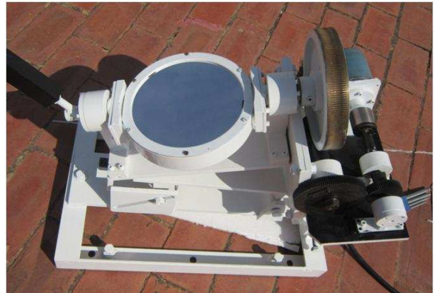
(left) WARM telescope auto-guider Lab setup. (right) Coelostat for Koaikanal outreach program.
