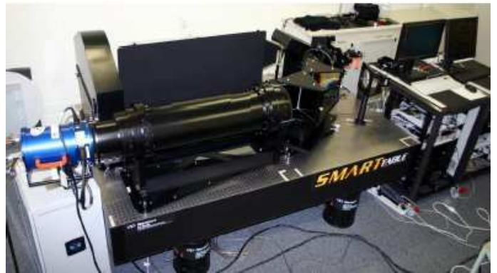
The Hanle Echelle Spectrograph with all its assemblies.
