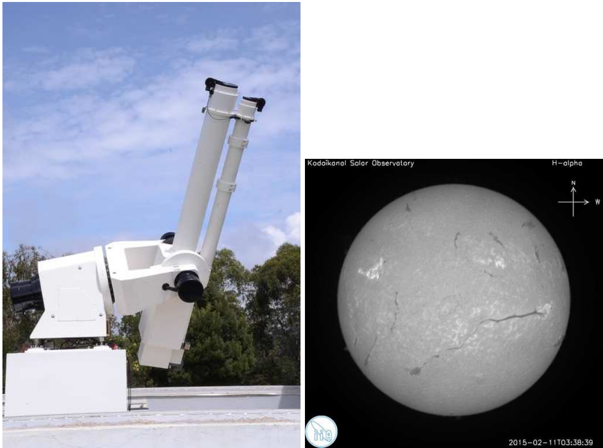
(left) H alpha Telescope at Kodaikanal. (right) An image obtained from H alpha telescope.
