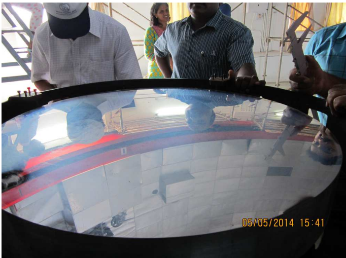
The secondary mirror of the VBT being removed for aluminisation.
