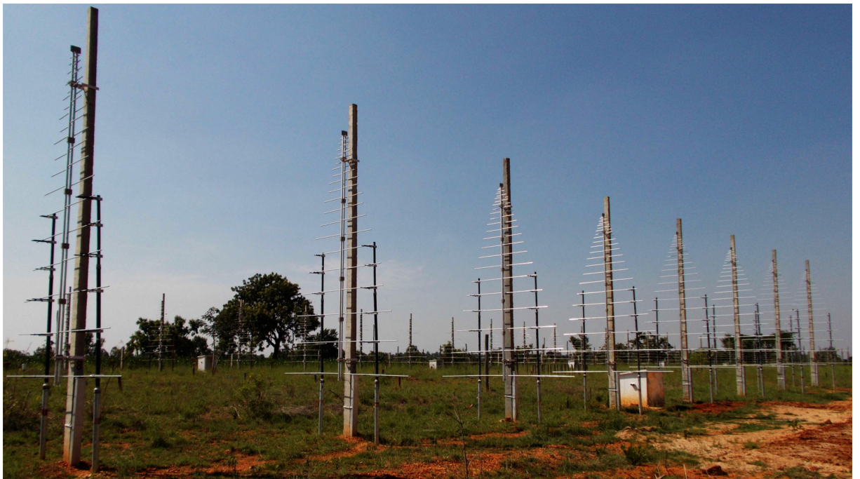
Figure 2.14: Photograph showing the front-end receiver system of Gauribidanur LOW-frequency Solar Spectrograph (GLOSS). Delay Shifter Boxes are protected inside the RCC box (a small cement housing seen at array center).
