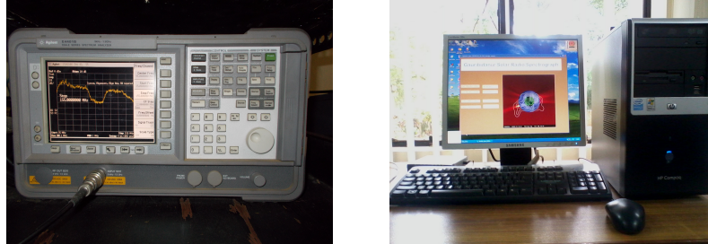
Figure 2.17: Left: The E4411B spectrum analyzer from M/s. Agilent Technologies that is used as the backend for GLOSS. Right: host PC with a PCI-GPIB interface that controls and stores the observed data with the spectrum analyzer.
