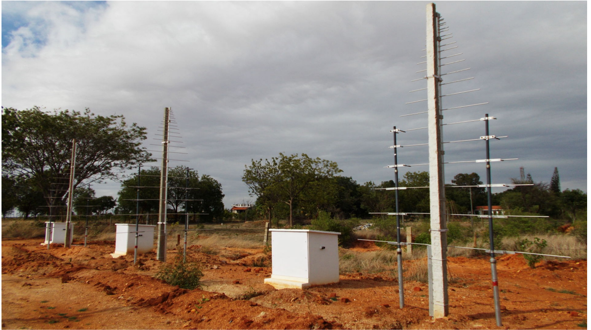
Figure 5.2: A view of the GRASP. The first and last LPDAs are in mutually orthogonal orientation, and they are part of the GRASP, the third antenna (middle) belongs to the e-CALLISTO set-up at the observatory [Benz et al. (2009)]. The “white” enclosures near each antenna house the respective RF-to-optical converter.
