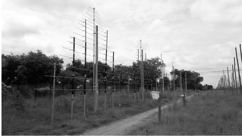
Figure 5.6: Image of a single group. The antennas are nearly 6m tall and 5m wide. The smaller antennas on the far side are a part of GRIP array.
