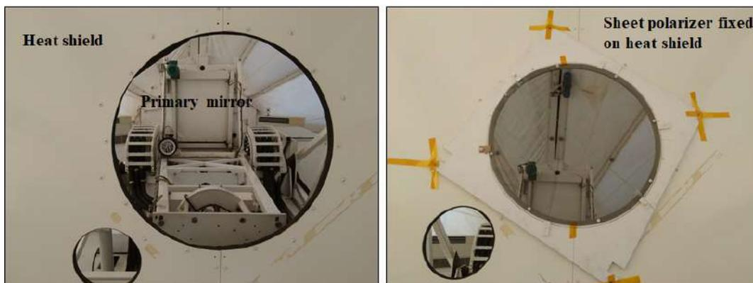
**Figure 7.6:** Sheet polarizer fixed on the heat shield of the telescope.
