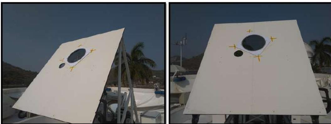
**Figure 7.7:** Telescope with sheet polarizer during the observations.
