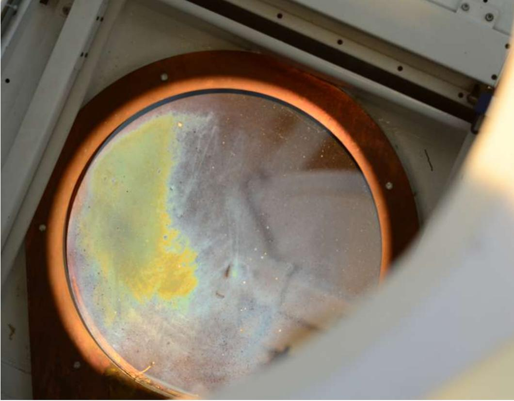
**Figure 7.11:** The coating degradation on the primary mirror during winter observations.
