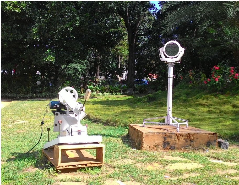
Coelostat used for observations of the solar chromosphere using narrow band imager at Indian Institute of Astrophysics, Bangalore
