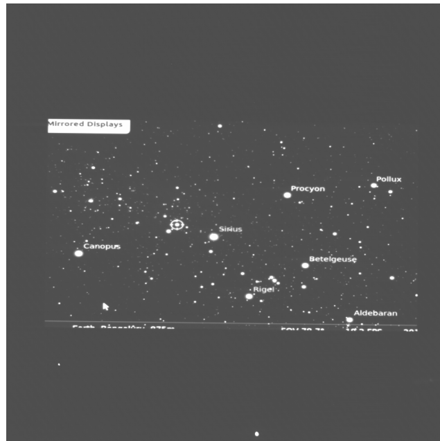
Figure 4.23: A Sample image captured from StarSense camera. A view of the software Stellarium was projected on a far away screen using an overhead projector. This image shows the capability of StarSense to focus on far away objects beyond it's hyper focal distance.
