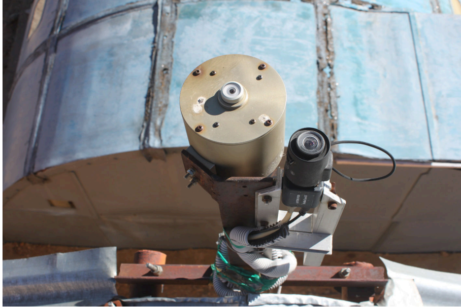
Fig. 4.1: CONCAM all sky camera installed at IAO Hanle along with StellaCam (black unit).
