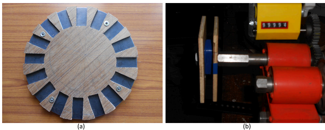
Fig. 6.2: (a) Plywood section attached to mild steel disk for fixing magnets, and (b) Rectangular bobbin made of plywood mounted on the coil winding machine.
