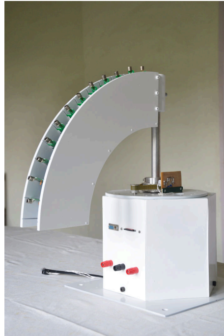
Fig. 4.5: Laboratory picture of the first version of the cloud monitor instrument.
