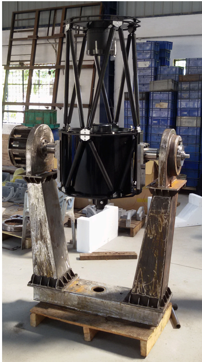
Fig. 5.22: Assembled MASS-DIMM telescope at the manufacturing facility. The azimuth drive unit is not yet completed, hence, not shown in the image.
