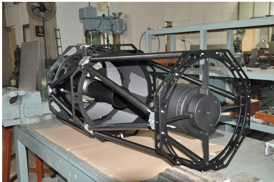
Fig. 5.7: TPO 16-inch F/8 Ritchey-Chretien truss OTA.
