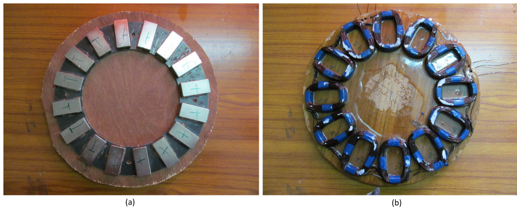
Fig. 6.1: (a) Rotor and (b) Stator unit of the Axial Flux Direct Drive motor.
