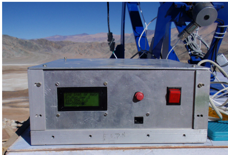
Fig. 2.13: Telescope Control System placed beside AEM, IP address of the instrument can also be seen on the LCD display.
