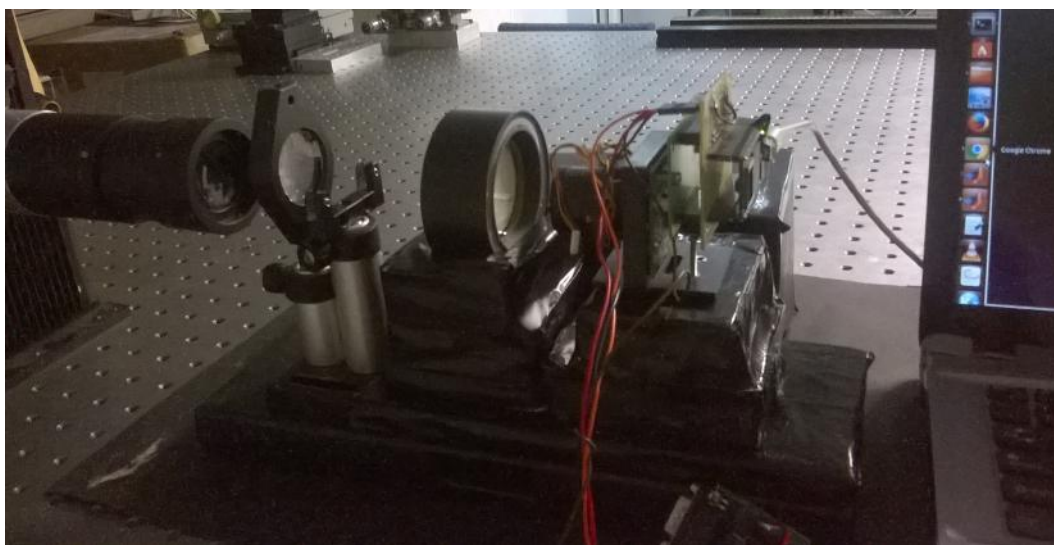
Figure 2.13: Detector test setup on the optical table. From left to right: UV light source, collimating lens, and the detector assembly with the MCP and the readout board.
