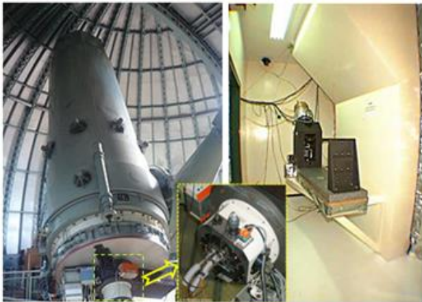
Figure 4: The 1.9m telescope at Haute-Provence Observatory in Southern France (Left panel). The ELODIE spectrograph credited with the discovery of 1st exoplanet was located in a separate room below the observatory floor (right panel). Fiber-pick up and calibration assembly attached to the Cassegrain focus of the telescope can be seen in the inset. (Image from: www.obs-hp.fr )
