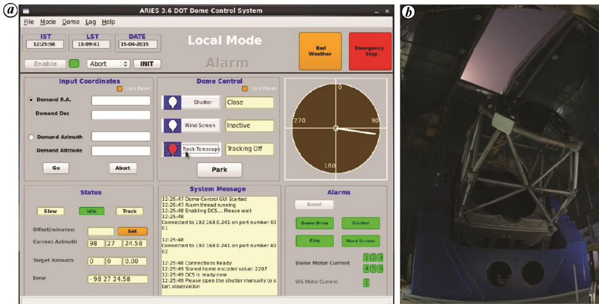
Figure 5. The software used for synchronization of telescope motion with that of the off-centred dome, designed and developed by ARIES. (a) DCS graphics user interface (GUI) and (b) telescope in synchronized position with dome to the right.
