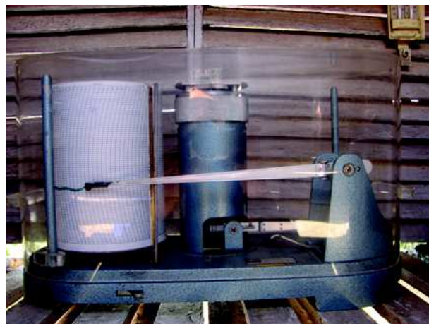
Fig. 6: Historical instruments for recording sunshine hours and pressure, those are operational at ARIES
