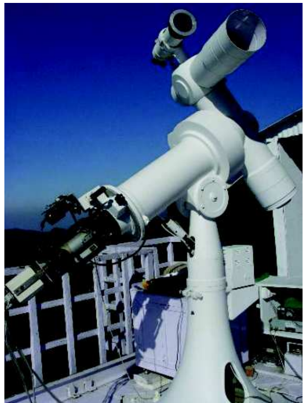
Fig. 23: 15 cm Coude tower telescope at ARIES
