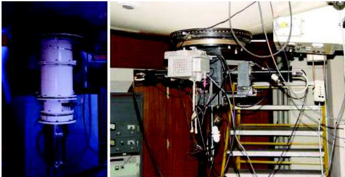
Fig. 30: The polarimeter (AIMPOL) and the Fast photometer mounted at the Cassegrain focus of the 104-cm telescope
