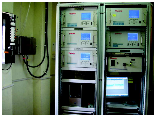
Fig. 8: Set of the instruments for O 3 , CO, NO-NO y , SO 2 operational (ISRO Environmental Observatories Project) at ARIES
