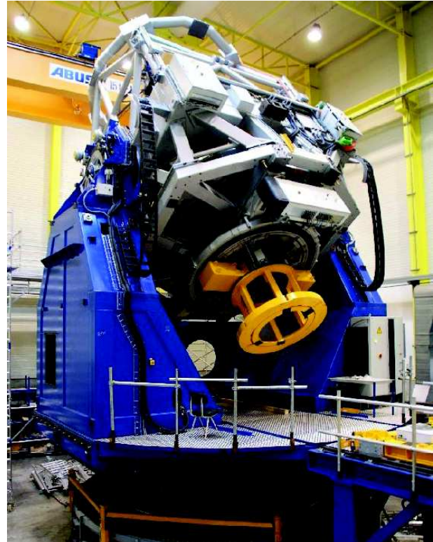
Fig. 40: A fully assembled 3.6m DOT in AMOS factory of Belgium
