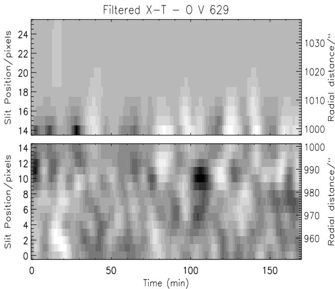
**Fig. 4.** X-T plot for dataset 26 438 showing the region between 14–25 pixels ( $\approx 1000$ – $1040''$ ), *top panel*, and the region between 0–14 pixels ( $\approx 950$ – $1000''$ ), *bottom panel*. The top panel image shows the square-root values of the flux, in order to enhance weaker features.
