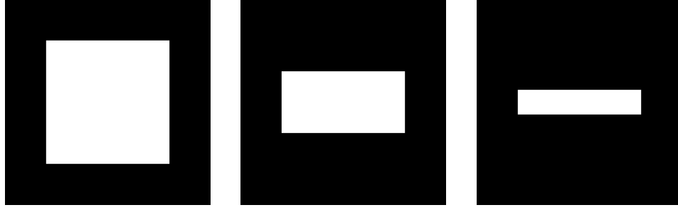
Figure 4.8: Images show rectangles, with sides p and q for p \geq q , for different aspect ratios, q/p . Left image shows square shaped structure which is isotropic. Middle image shows a rectangular shaped structure with aspect ratio of 0.5. Rectangular structure with aspect ratio of 0.2 is shown in the right image.
