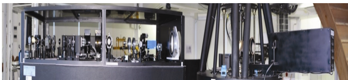
Figure 5. The back-end instruments on an optical bench, including the AO, narrow-band imager and polarimeter.
