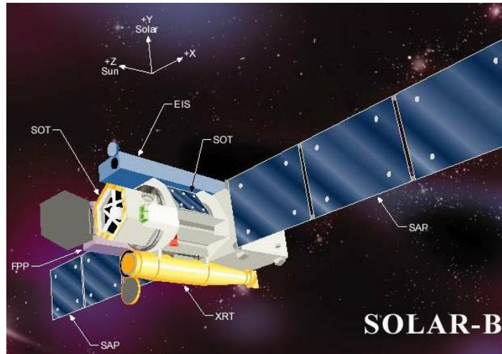
FIGURE 2.4: Hinode spacecraft with the positions of the instruments SOT, EIS and XRT. Image credit: JAXA
