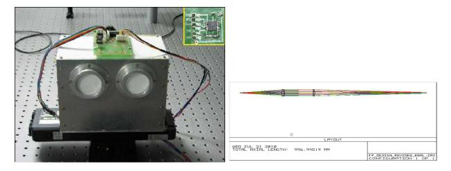
Figure 2.28: Left: A picture of the dual window filter oven and the temperature controller unit. The whole unit has been kept on the translational stage for selecting one window at a time during the solar observations. Right: The optical ray tracing obtained from Zeemax software.
