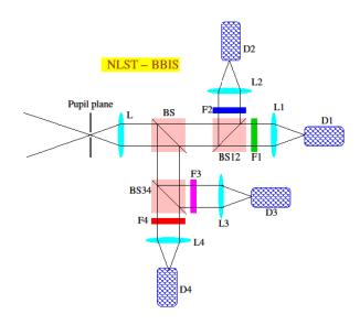
Figure 2.26: Concept design of NLST Broad Band Imaging System. L denotes lens, BS - Beam splitter, F - filter, D - CCD.
