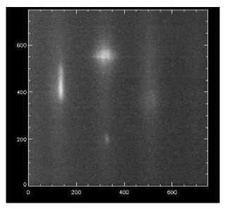
Figure 2.32: The multi-slit spectra in the green emission line at 530.3 nm obtained during the total solar eclipse of July 11, 2010 from Easter Island covering a field of view (FOV) up to about 2 solar radii. The use of narrow band interference filter of about 0.3 nm FWHM permits to record 3 spectra due to three slits each separated by about 1.1 solar radii. Emission lines are seen against the weak background continuum.
