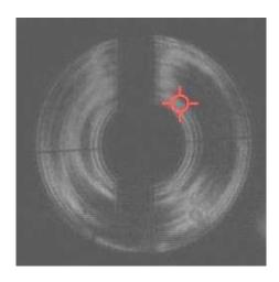
Figure 2.7: Ronchi gram of the integrated system.
