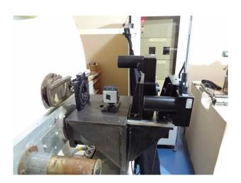
Figure 2.2: Rotation stages of the polarimeter at Solar Tower Telescope.
