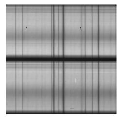
Figure 2.29: A typical spectropolarimetric observations of the magnetically sensitive 6302 ÅFe doublet line wavelength region taken with the newly automated polarimeter at the Kodaikanal tower telescope can be seen in this figure. The Fe lines seen here are considerably broadened across the faint Sunspot region. The central dark patch denotes the separation between the two beams which are orthogonally polarized to each other.
