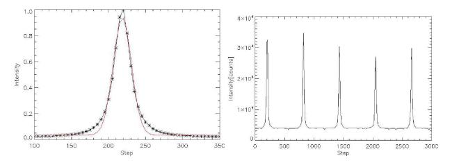
Figure 2.27: Left: The average intensity profile of one transmission peak (black curve). A Gaussian fit to the measured intensity profile (red curve). The wavelength is shown in discrete steps of the CS-100 controller. Right: A transmission profile of the Fabry-Perot etalon. The X-axis is shown in terms of discrete steps of the CS-100 controller.
