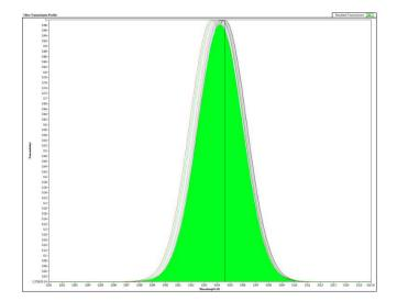
Figure 2.31: Number of curves show the shift in the transmission of the filter as a function of the incident angle of the beam. The curve enclosing the area shown in green represents the average curve of the transmission through the filter.
