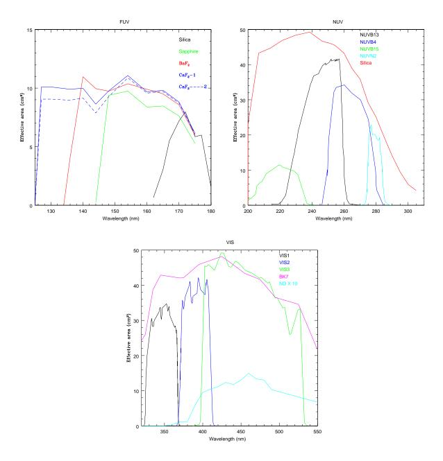
Figure 2.23: Effective apertures are shown for all the filters.
