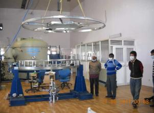
Figure 2.1: Left: The process of removal of the existing aluminium coating on HAGAR mirror. Right: Loading of the HAGAR mirror into 2.5 m vacuum coating chamber at Hanle.
