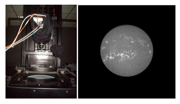
Figure 2.4: (Left) The high resolution digitizer with light table and CCD camera (Right) Sample calcium K filtergram digitized and calibrated.
