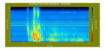
Figure 2.15: Dynamic spectrum of the transient radio emission from the Sun observed with the GRASS in the frequency range 35-155 MHz. The horizontal lines of intense emission over the 90-110 MHz band are due to radio frequency inteference (RFI) related to FM transmission from Bangalore. The intermittent emission around 120 and 140 MHz are also due to RFI, All-India Radio broadcast.
