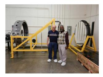
Figure 2.6: The optics test setup with primary at left in its cell and flat mirror at right. The secondary mirror in its ring mount is hidden behind the persons in the picture.
