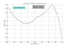
Figure 2.8: Global wavefront error of the system (3 surfaces, double pass).
