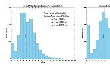
Figure 2.24: Histograms of distribution of r0 at height of 26 m at Hanle and Merak sites, from SHABAR results.
