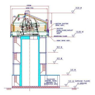
Figure 2.12: Schematic section of telescope enclosure and dome. The telescope is shown mounted atop the hallow pier. The telescope mirror can be lowered down through the pier for aluminising
