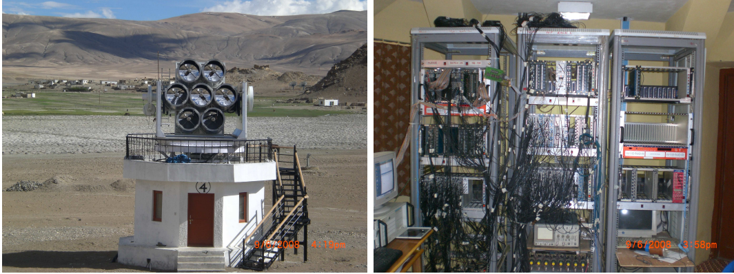
Figure 2.15: An image of a single telescope of HAGAR array and backend electronics
