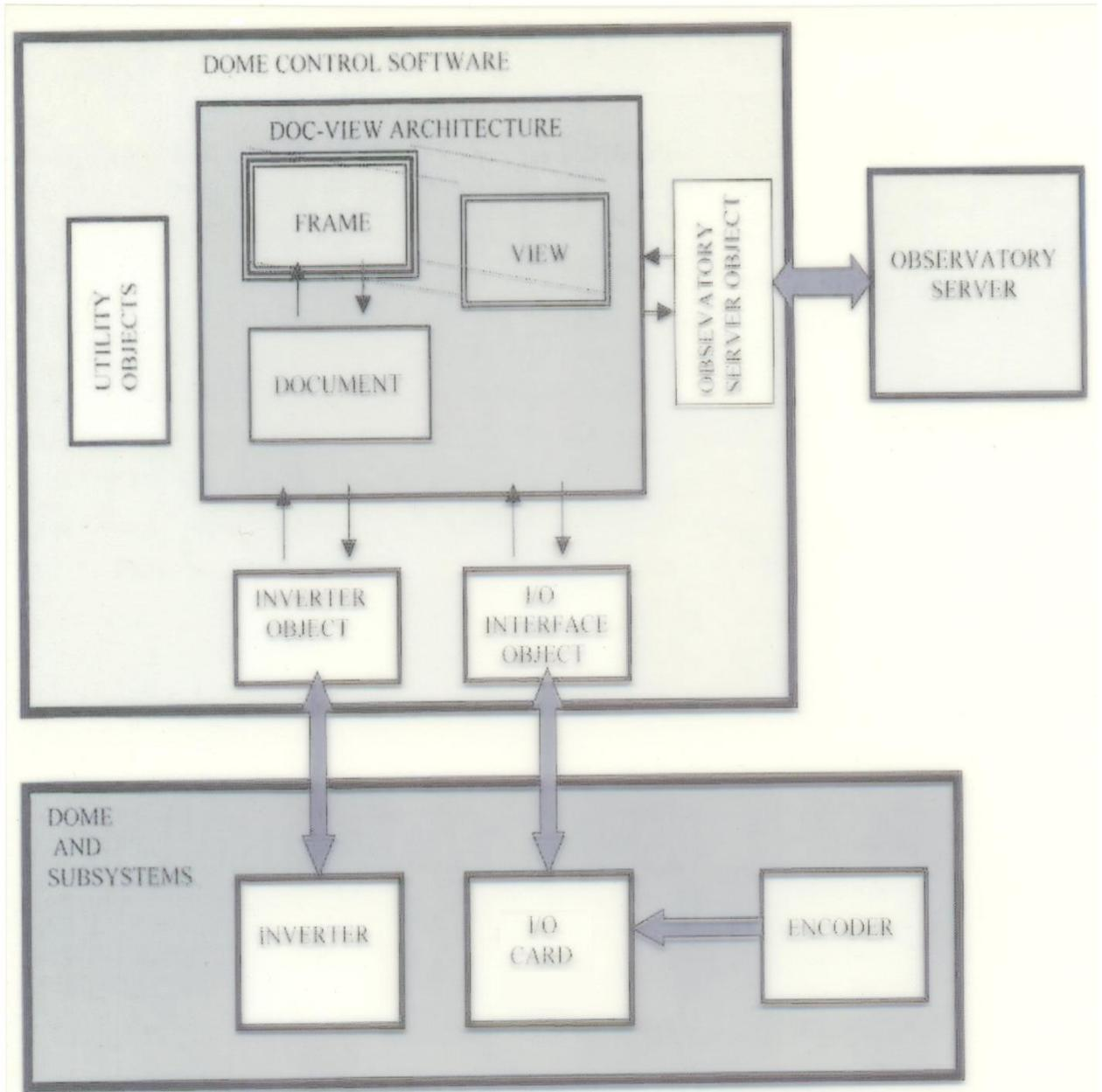
Fig( 2): Software Control Scheme
