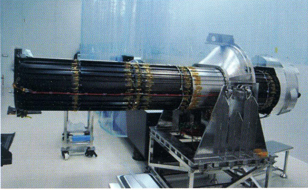
Fig. 2. EM of UVIT at the MGKM lab, CREST, IIA, Hosakote. View of main Baffles and telescope tubes of NUV channel.
