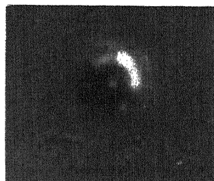
Fig. 1. Shapes of the fringe pattern taken using a 3-hole aperture mask, with a narrowband filter centred on \lambda 5577 Å and FWHM 100 Å. The aperture was arranged in a triangular pattern.
