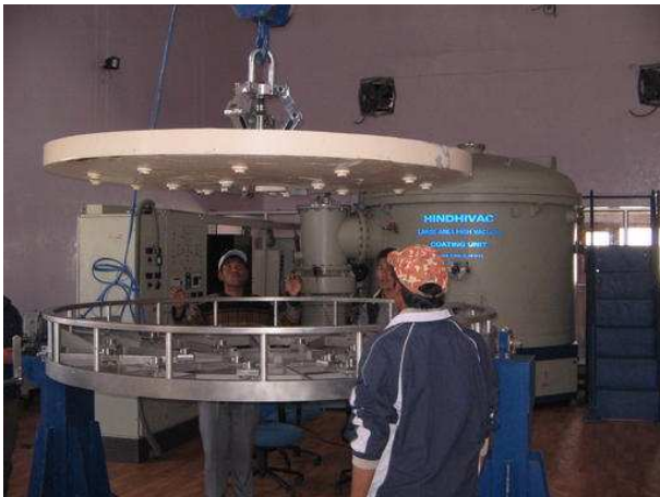
Figure 2.8: Dummy mirror being loaded on to the tilting fixture.
