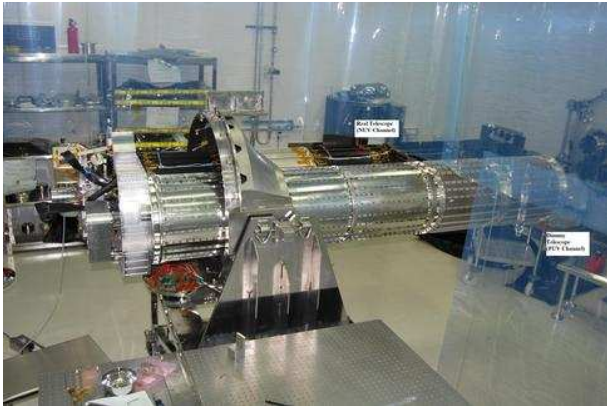
Figure 2.23: Engineering Model (EM)-UVIT Payload in class 1000 area at CREST, IIA. In EM-UVIT is shown: NUV/VIS (black colour), telescope is identical to Flight Model (FM), and the other telescope is a mass equivalent of FUV telescope.
