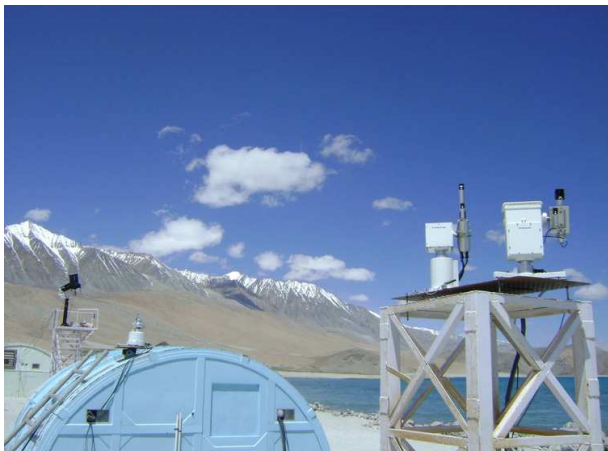
Figure 2.26: Sky radiometer installed at Merak on a 3m tower, beside the observing hut. The IIA-SDIMM on a 4m tower is seen in the background.
