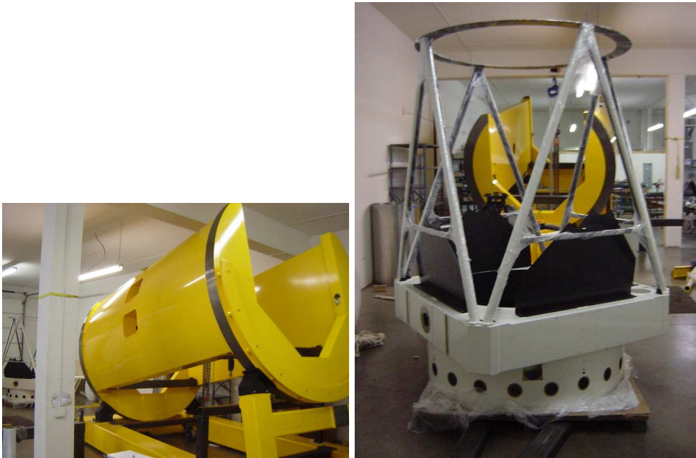
Figure 2.12: The assembled mount of the 1.3m telescope at the vendor facility
