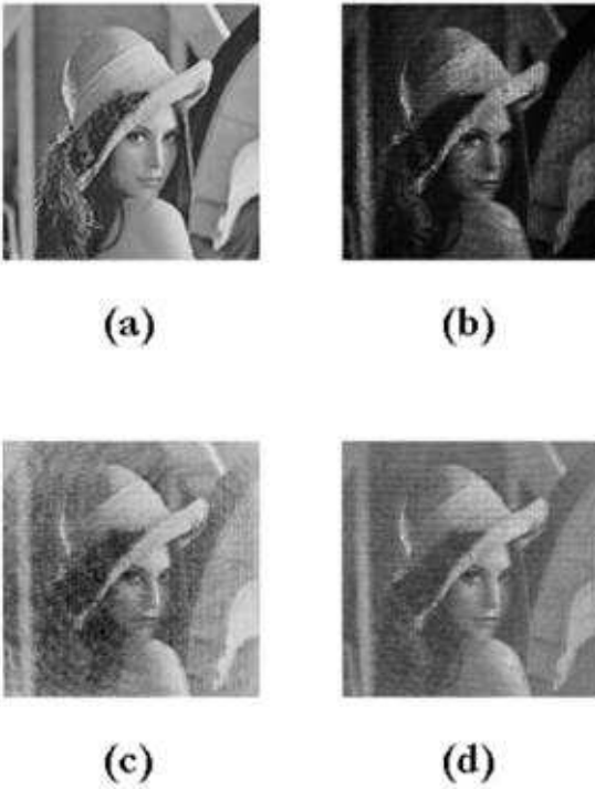
Figure 1.39: (a) Actual image, correlation coefficient ( c = 1.0000 ) (b) Image captured by the CCD, c = 0.6778 (c) Resultant image after simple subtraction of bright background, c = 0.6146 (d) Image obtained after subtracting the dark background, c = 0.7121 .
