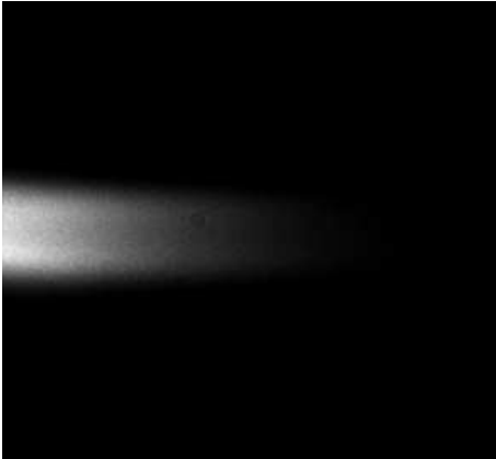
Figure 1.3: A representative H-alpha image: A slit width of 300\mu at the East limb of the sun was used with an exposure time of 126 ms at 7.1 Hz.
