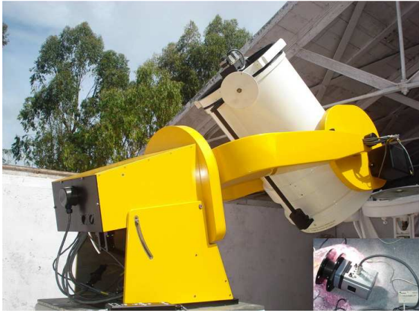
Figure 2.10: The newly installed 40cm DFM telescope at the Kodaikanal Observatory. Inset is the picture of the adaptor for G-band filter and the CCD camera.
