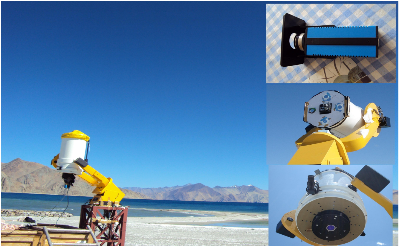
Fig-1. Main frame: The 16" classical Cassegrain telescope is installed at the shores of Pangong lake near Merak village on a robust platform at a height of about 1.63m from the ground surface. A high resolution PCO 2000 imaging camera (bluish in color) is also seen at its back end. Top right frame: PCO camera and its black anodized adapter. Middle right: Affixed 3.8 ND filter in the four holes of the aperture. Bottom
