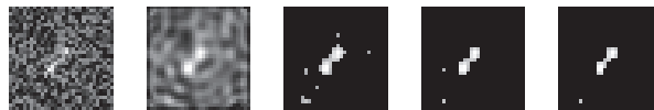
Fig. 20. The first row contains spots ( 32 \times 32 pixels) with \text{SNR} = 1, 2, 3, 4 . The second row contains spots reconstructed using Zernike moments with n \leq 24 . The third row contains the thresholded spots with intensity greater than 60% of maximum intensity.
