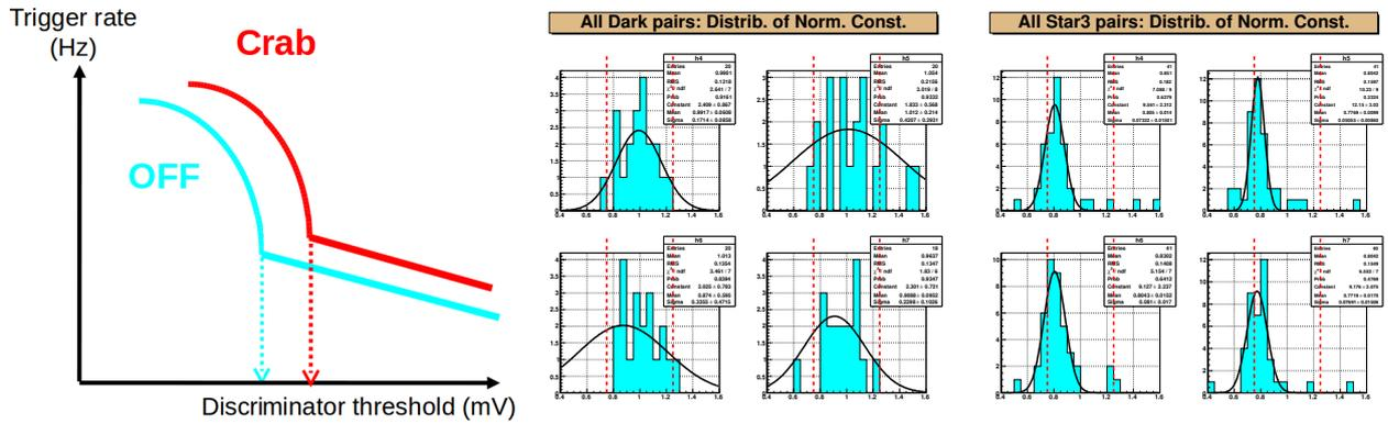
**Fig. 1.** (a) Representation of the Crab ON/OFF trigger rate versus hardware energy threshold. (b) Distribution of normalisation constants “C2” for “dark regions”. (c) Distribution of normalisation constants “C1” for “star3” runs. From left to right and top to bottom of (b) and (c) respectively, are normalisation constants for NTT=4, 5, 6 and 7. The dashed red vertical lines delimitate the accepted range of C for dark region pairs (Paper I).
