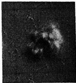
Fig. 1 Speckles of the artificial star image obtained in the laboratory using a filter centered on 5577A (FWHM 100A).
