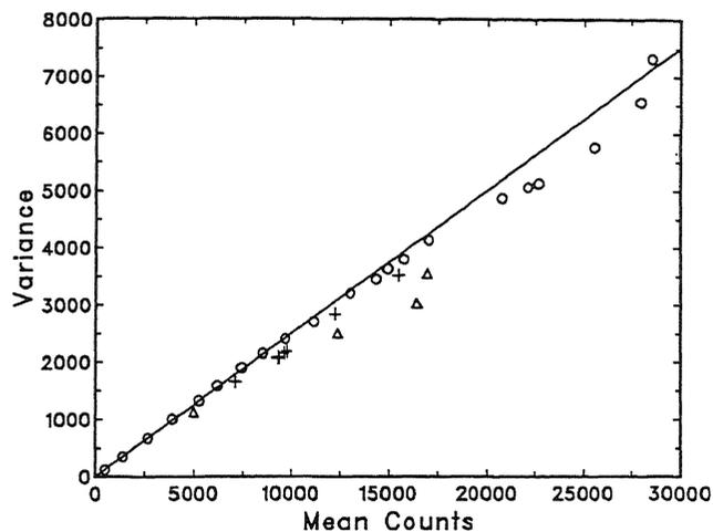
Figure 1. The variance in observed counts as a function of mean signal counts. Circles represent results based on 21 flats recorded in the laboratory. Other symbols represent results based on a smaller number of dome flats obtained at the prime focus of the VBT. The straight line is the fit with a read-out noise of 8 electrons, and a system gain of 0.25 counts per electron, or  $Q = 4$  electrons per count.
