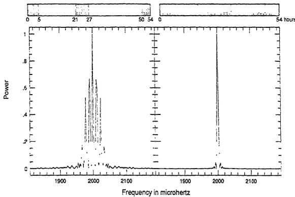
Fig 1. Fourier transforms of a single, noise-free, un-tapered sine wave sampled as indicated at the top of each panel. Fig 1a (left panel) shows the "alias" pattern typical of time series data from a single site with daytime gaps. Fig 1b (right panel) shows the pattern obtained if the gaps are not present.
