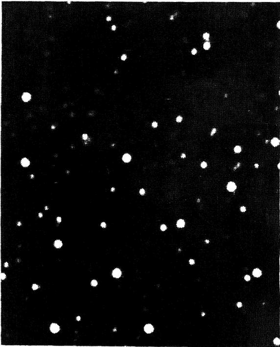
a 3 x 3 binning. This essentially degrades the image to the equivalent 2 arc second seeing images. The figure above shows a typical frame of the image acquired in the scan mode. The effective exposure time is 24 seconds. The limiting magnitude is about 20.5.
