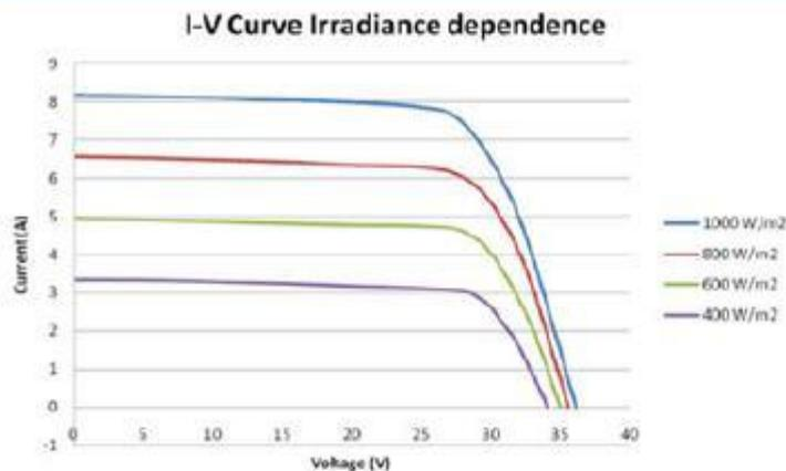
Current/voltage characteristics with dependence on irradiance tested at AM 1,5 and 25°C
