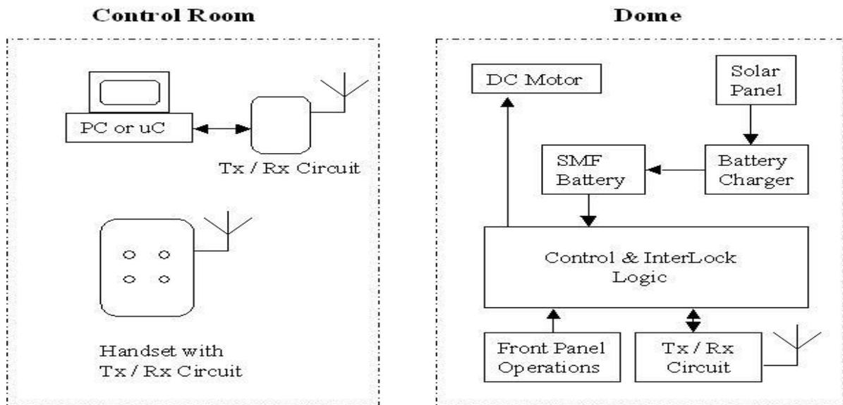
Fig 1 : Control Schematic
