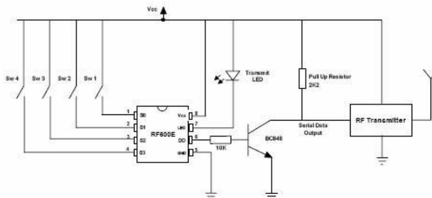
Not that a circuit constructed using AM radio modules does not need to have transistor BC848, resistor 10K or 2k2 Pull up resistor fitted.
