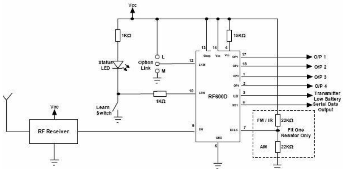
This circuit provides a complete decoding solution capable of learning up to 7 unique encoders
