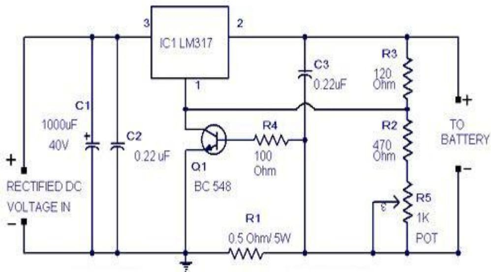
Fig 3 : Simple Lead Acid Battery Charger using LM317.
