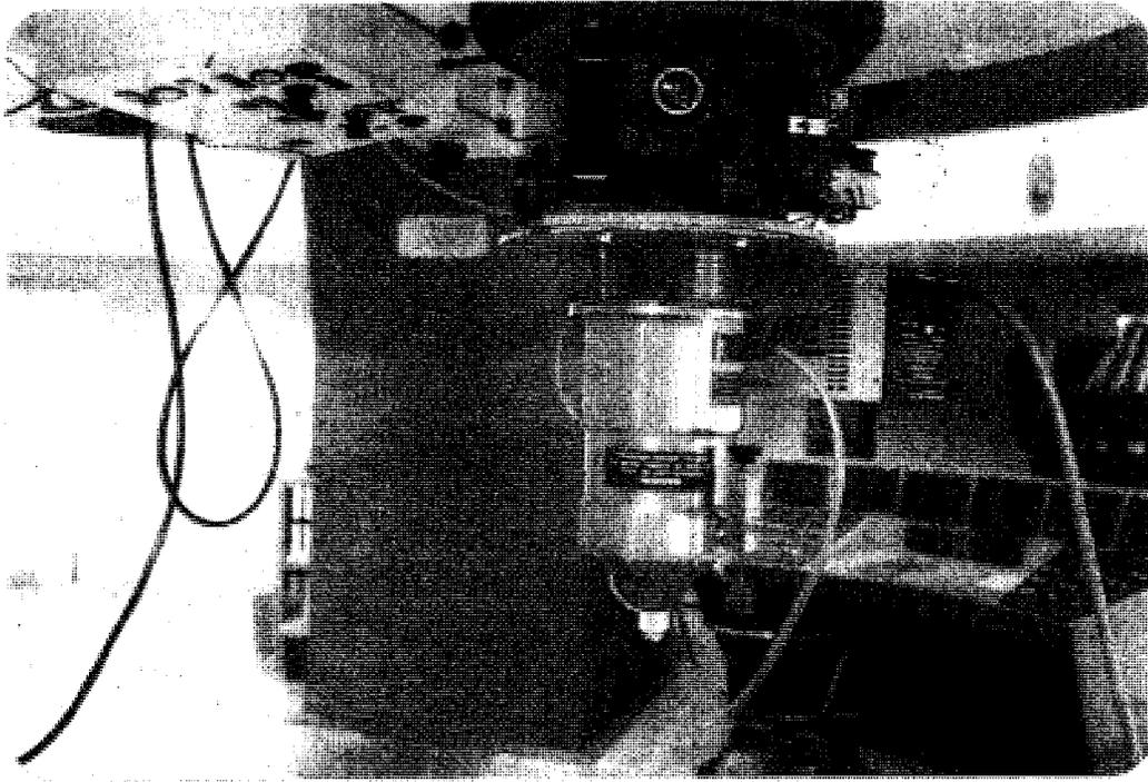
CCD System mounted on the 1 m telescope at Kavalur.
