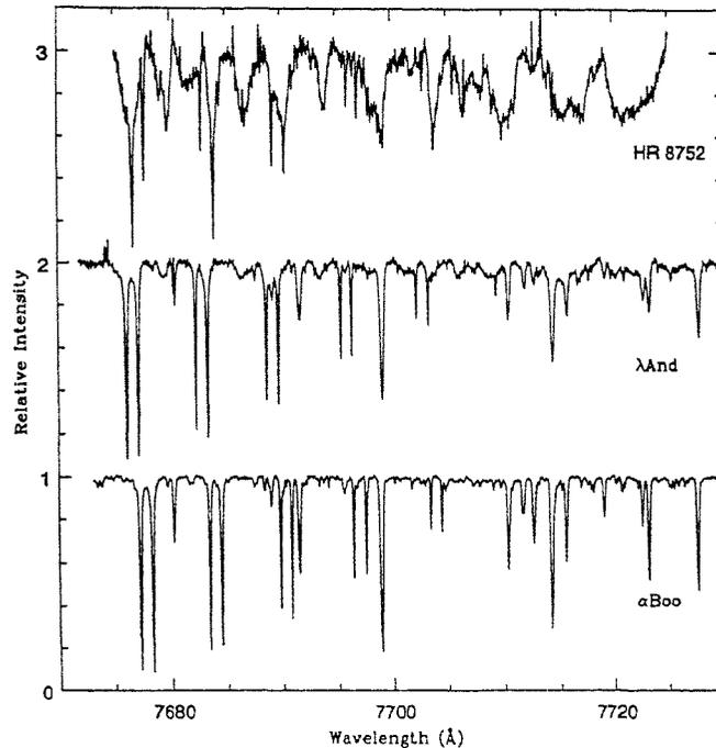
Figure 8: Spectra of three stars in the region of KI,  $\lambda$  7699 with VBT echelle spectrometer. The spectra taken due to terrestrial  $O_2$ ; the width of stellar line changes in the three objects.
