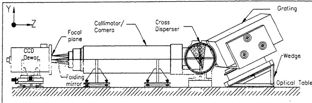
Figure 1: Optomechanical layout of the Spectrometer. F/5 beam emerging from the slit fed into the collimator by a folding mirror. Then the collimated beam passes through the cross disperser (prism) and get pre dispersed and then illuminates the echelle grating. The dispersed beam from the grating again passes through the prism second time and finally comes to focus on to the CCD plane where the spectrum is recorded.
