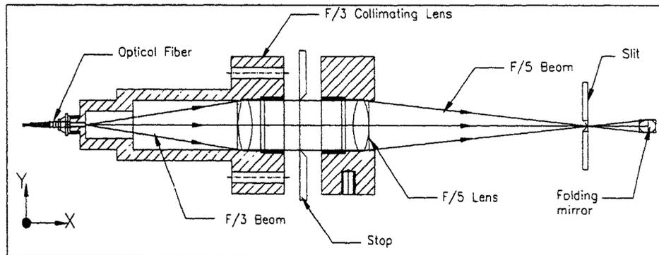
Figure 2: F-Ratio enlarger. F/3 beam from the optical fiber is converted into a collimated beam by the F/3 collimating lens then it is re-converted into F/5 converging beam by another F/5 lens. The slit positioned at the focus of the converging beam. The beam diverging from the slit falls on the folding mirror which redirects the beam into the spectrometer collimator.
