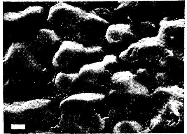
Fig. 1: Close-up view of "large" perovskite crystals intergrown with second-generation spinel. Perovskite is partially overlain by submicron spinel which must have formed after the perovskite had grown on the parent spinel. Scale bar 1 micron.
