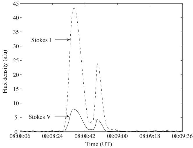
**Figure 4.** Time profile of the Stokes  $I$  &  $V$  emission observed from the Sun around the same time as the radio bursts in Figures 1 and 3, on 2009 May 8 at 77 MHz. The integration time is  $\approx 1$  s. The estimated dcp of the transient Stokes  $V$  emission, present immediately prior to as well as after 08:08:42 UT, is  $\approx 0.18$ .
