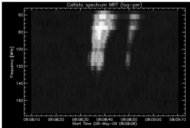
**Figure 1.** Dynamic spectrum of the two type III radio bursts observed with the CALLISTO radio spectrograph at Mauritius on 2009 May 8 during the interval 08:08:35–08:08:55 UT. The sweep time is  $\approx 200$  ms.
